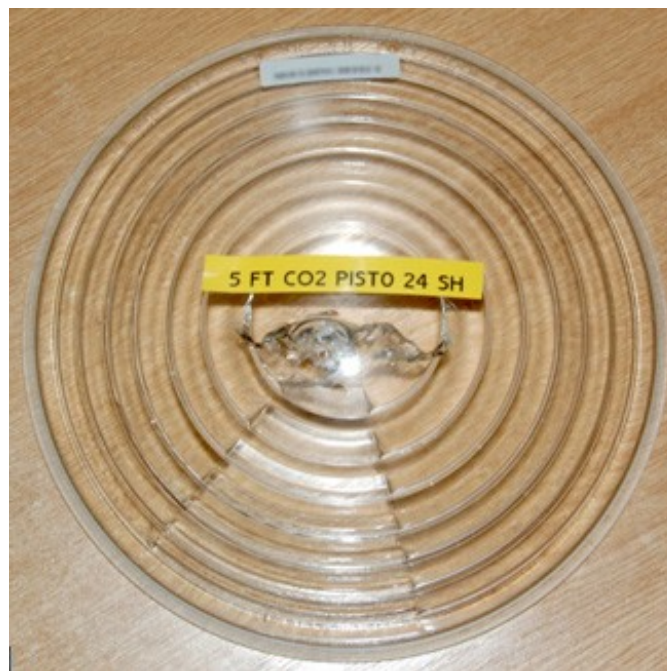
Glass Lens B damage after 24 shots at 5 foot from a Pietro CO2 4.5mm 117 Cal Beretta 92 MOD FS
